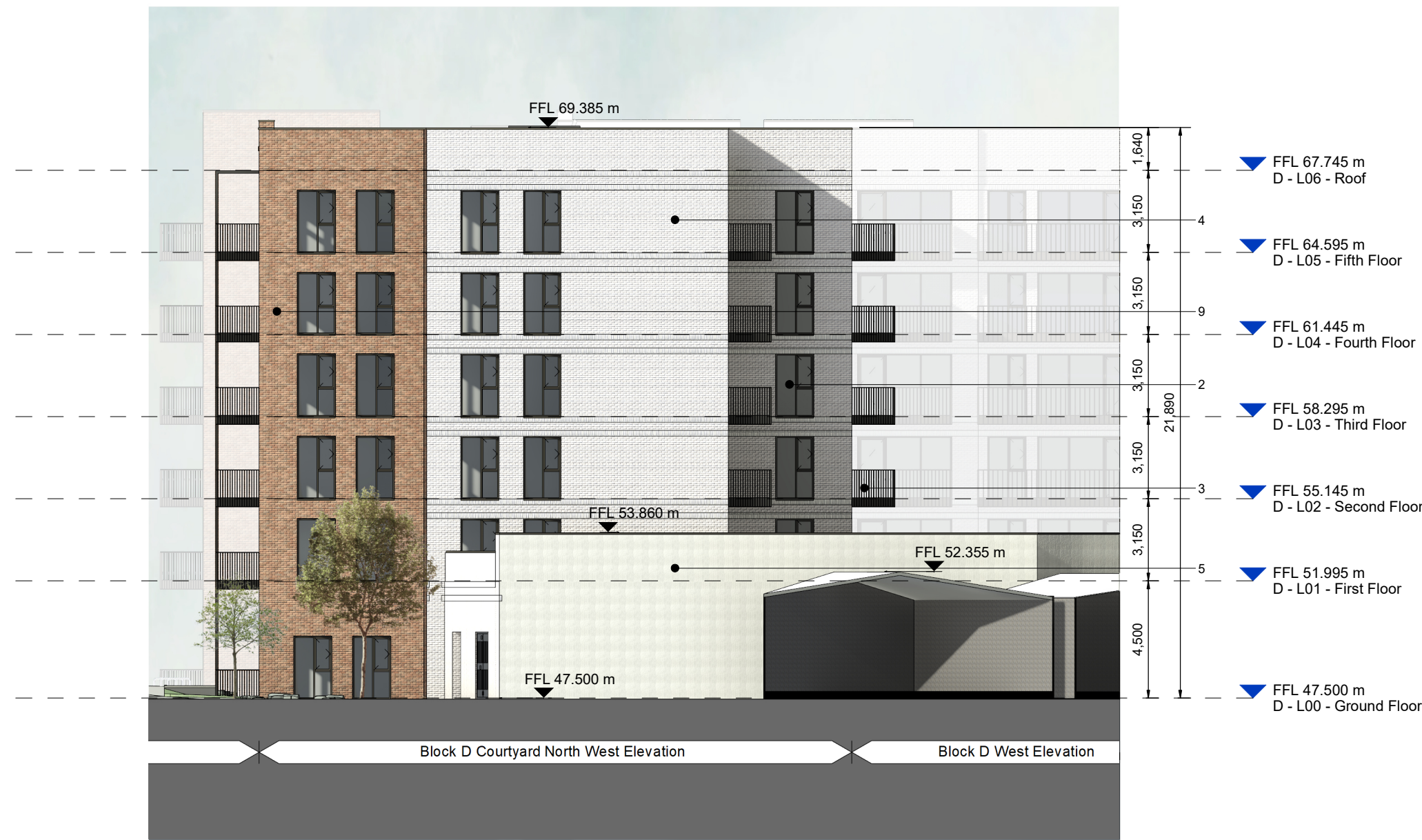
Blocks D, Planning Permission, Elevation North West 1 : 200
