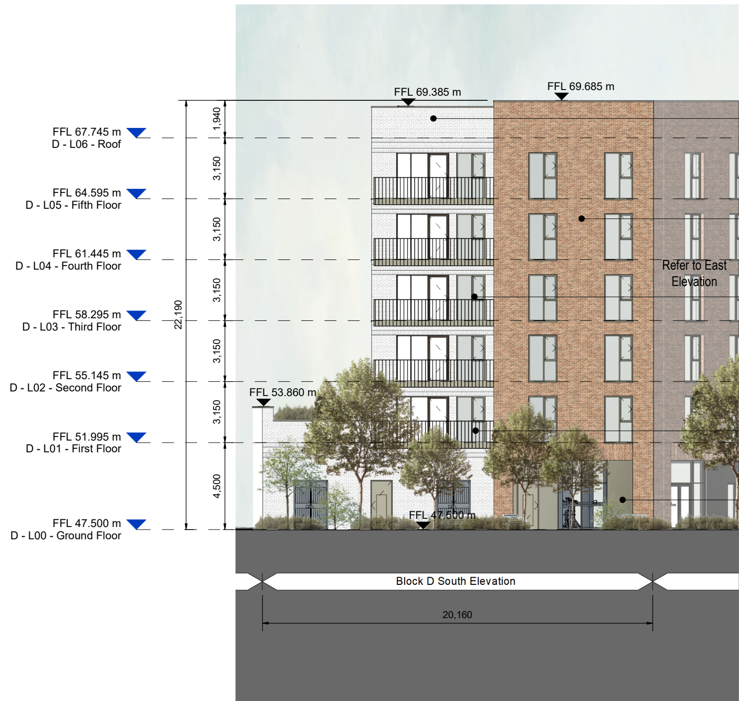
Blocks D, Planning Permission, Elevation South 1 : 200
